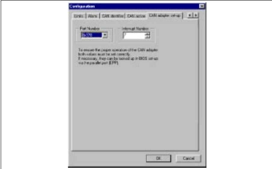
Fig. 7-22 Parameter setting: Dialog box Configuration , Menu CAN adapter set-up
